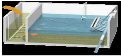
**Decant Phase** – The decanter descends gradually downward to draw off the clarified supernatant. Wastewater continues to flow into the prereact zone as the treated and clarified effluent is decanted from the main react zone at a constant rate. Waste activated sludge is typically removed from the basin during this phase.
