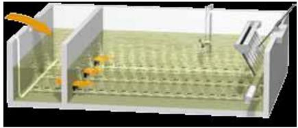
**React Phase** - Here screened wastewater flows continuously into the pre-react zone and enters the main react zone through submerged ports in the baffle wall.
