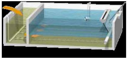
Settle Phase – Basin agitation from react phase (i.e. aeration and mixing) is stopped to allow the solids to settle to the bottom of the basin. Raw wastewater continues to flow into the pre-react zone while the main react zone settles. As solids settle, a clear layer of water develops on the top of the basin.
